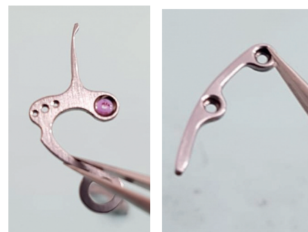
Just two of the many individual chronograph parts being re-finished.
