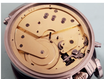
The dial side half stripped down to check the movement fits into the case properly and that this side setting adjustment for changing the time is correct.
