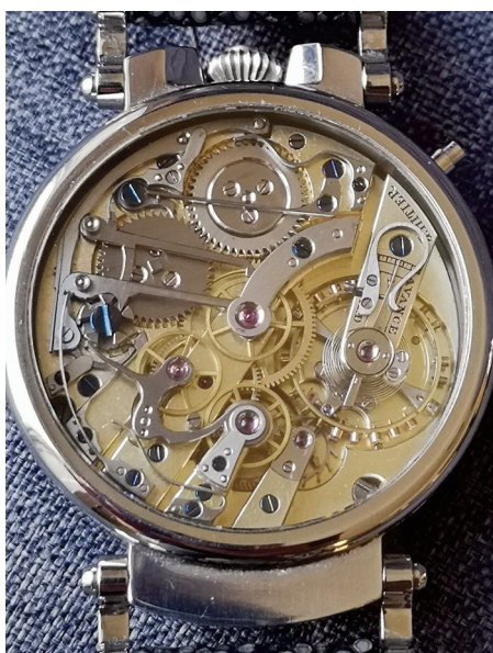
The clear sapphire caseback, both sapphire glasses have been UV treated to stop moisture condensation.
