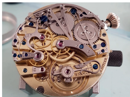
The movement complete with polished/blued screws and temperature compensating balance.
