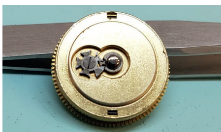
The barrel complete showing its Geneva (Maltese Cross) stop work.
